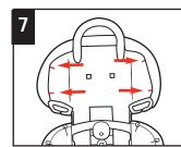
From the back of headrest, pull pad out from behind the pad locking tabs
